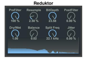
Decimates and reduces the bit depth of your signal. It is dual band, i.e. the reduction can be applied only to a portion of the signal.
