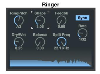
A dual band ring modulator with distortion and delay with feedback.
