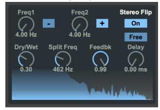
A dual band frequency shifter with feedback delay
