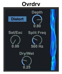
Ovrdrv is a distortion device: it goes from very subtle to total destruction. It can operate on the signal below (Saturation) or above (Excitation) a given frequency.
