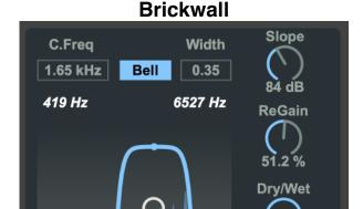
A band-pass/band-reject brickwall filter; the slope can go up to 192 dB of attenuation per octave (in other words it can be extremely selective)
