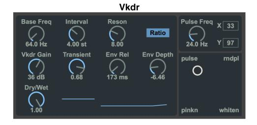
This is a vocoder effect. Not to be confused with the "phase vocoder", the vocoder is a filter effect which analyses a signal and recreate it using a broadband source (for instance a white noise) and a bank of filters.
