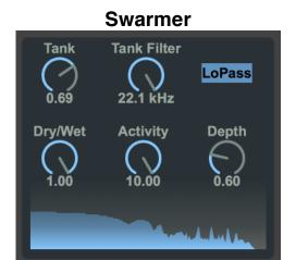
A "superchorus", excellent to create super fat synth sounds (and more). It is composed of a chain of modulated delay lines.
