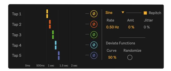
As well as having additional features, this panel visualizes the taps delay time when its modulated. The two blocks with the same color on each row represent the L/R channel of that delay line.  $\varnothing$  toggle on each tap inverts the polarity to negative
