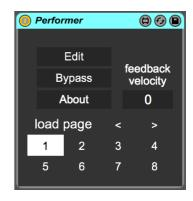
By activating the "Bypass" button, the device won't react to any input. That way you can use the controller for other purposes and don't have to worry about triggering the animations. When editing an animation with the Frame Editor the Performer will also automatically activate the bypass mode. Then you can draw on this controller without playing back animations at the same time.
