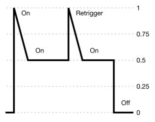
A trigger signal can be in 3 different states: 0, 0.5 and 1.
