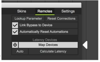
In order to compensate for it correctly, Modulat has to calculate the latency of your project, which you can do by pressing the "Calculate Latency" button below.
