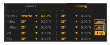
The *Routing* tab is where you map modulators to destinations. Each modulator has 2 destination options each with a bipolar attenuator. In additon to the two LFOs and envelopes, there are two random *Spray* values (which are create at the beginning of each voice), the input audio's envelope follower and pitch
