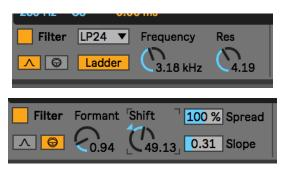
There are several filter options. By default is a simple biquadratic filter, with a *Ladder* filter options and shapes. Additionally, there is a *Formant* filter mode in which you can select the *Formant* (a tenor-alto blend I made), *Shift* their center frequencies, adjust their *Spread* and *Slope* adjusts their bandwidth.
