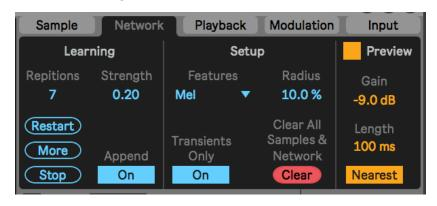
Here is where you manage the SOM neural network. On the left are parameters for training the network. There is the number of *Repitions* that the network does each time a new training is triggered. Each repetition every transient or spectral frame of the sample is fed into the network. *Strength* sets the amount the network
