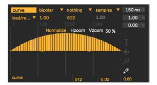
**guass** - Like curve, gauss show on the top the speed limit update rate and only a "Gaussian standard deviation" parameter.
