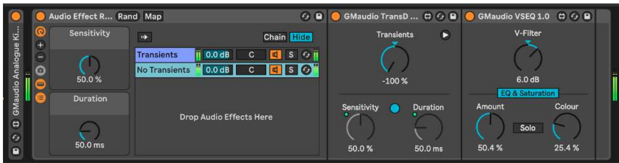
Example Device Chain using TransD 2.0 for processing different parts of the sound independently
