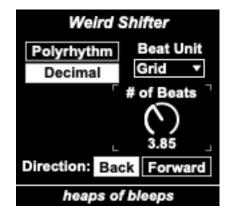
The "Weird Shifter" MIDI tool allows you to rhythmically shift your MIDI along non traditional polyrhythmic, polymetric, tuplet, and non dyadic grids.
