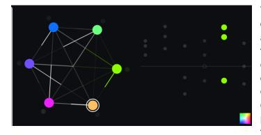
The top center of the device has two displays, one for the markov chain (left) and the other for the pitch transpositions for each chord (right). For the markov chain, each colored circle represents a different chord. Each circle has lines coming out of it and pointing to other circles. These lines represent the probability that the chord will transition to the chord that the line is pointing at.
