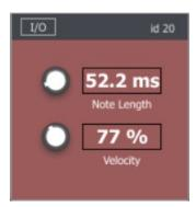
This device will trigger a second note from the note off message. The note length can be set, and velocity can be set relative to the original note.
