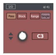
This device will filter the midi notes based on the pitch. It can be set to allow or block a specific range of midi values or a single value. Again this could be used to simply trigger a parameter change using a specific note or range of notes.
