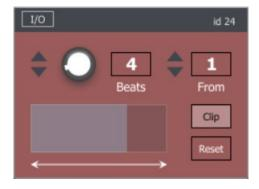
This is one device that actually uses Live's transport, and will open and close the gate based on a proportion of a sequence length in beats. Changing the slider to open the gate for different lengths of time on the fly can make for some easy live note filtering. This one can also be set to reset on the beginning of a looped clip.
