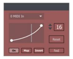
Incoming midi notes are used to trigger increments in parameter changes. The number of notes used to go through the whole sequence is set with the number box. The device can go forwards and loop or it can be set to palindrome mode where once the maximum is reached it will go in reverse and loop like that.
