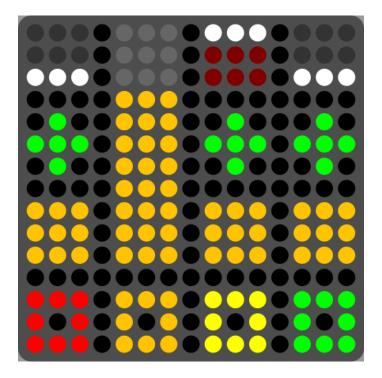
Mod CC allows the user to build a custom MIDI controller which has 12 customizable slots and 4 sliders. Each slot can hold a switch, pressure pad or a momentary button. Along the bottom row are buttons which open and close a slider, which will open in that column. When the slider is hidden, the colour of the button reflects the value of the slider from green to red.
