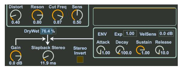
After the filtering the signal is shaped by an **Amplitude Envelope** (the frame on the right) wich has an **Exp** parameter (to get exponential segments) and a **VelSens** (Velocity Sensitivity) parameter expressed in dB.
