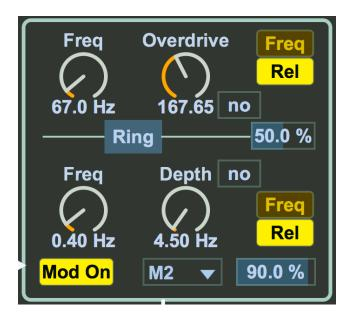
Oscillators 3 and 4 are joined in a Ring Modulation circuit. Moreover the fourth oscillator is frequency modulated by the first two oscillators.
