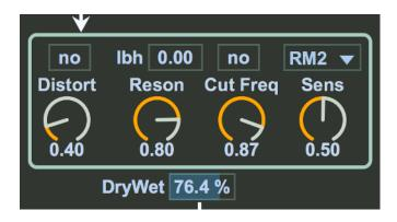
In this section the signal is first distorted using an algorithm not used in the oscillators distortion (parameter **Distort**), then sent to a 24 dB "morphing" filter. Note that the **Distortion** parameter can be modulated by the **LFO/Envelopes** modulators.
