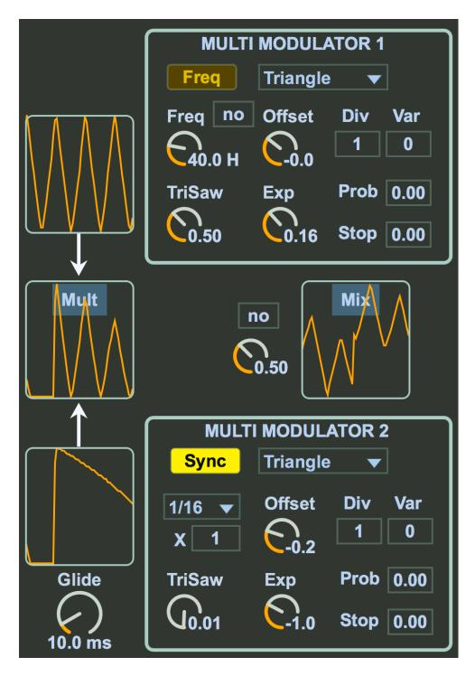
There are two **Multi Modulators**, which are a series of different *unipolar* (i.e. only positive) oscillators with parameters to change their shape.
