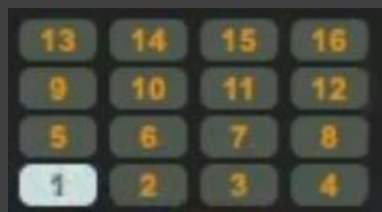
Fig 5: TheFade offers 16 slots for storing Fade patterns which can be triggered by MIDI notes or by clicking each number.
