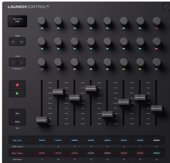
DAW Mixer Mode — encoder rows 1–2 sends, row 3 pan; buttons Solo (upper), Arm (lower)
