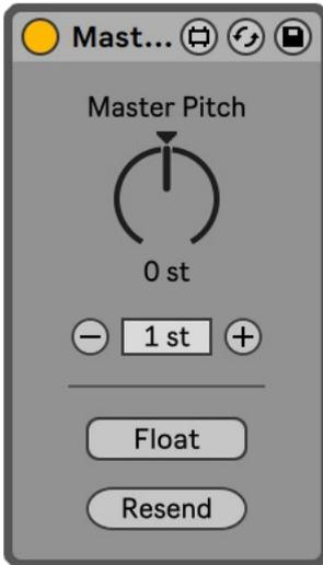
This is the master device that controls the other devices. It sends the transposition value that the other devices (Track, Device and Map) will use. It can be placed on any track, although it is most convenient to place it on the Main track. It can be displayed in a floating window using the Float button (which can be mapped)
