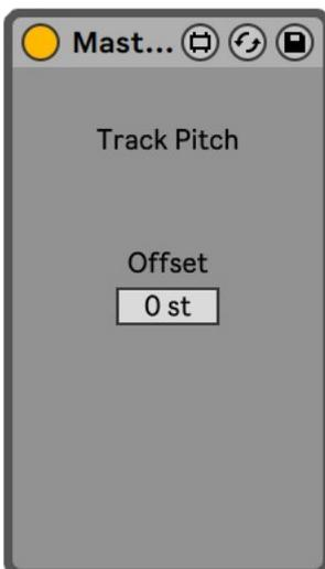
This device transposes MIDI notes that pass through it. It is designed for use on MIDI tracks. The most common place of use is at the beginning of the track's effects chain.
