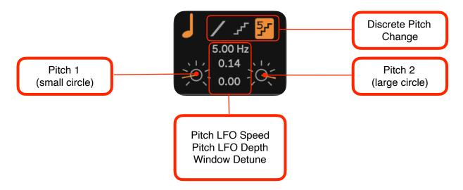
Pitch 1 & Pitch 2 Controls pitch for small and big delays.
