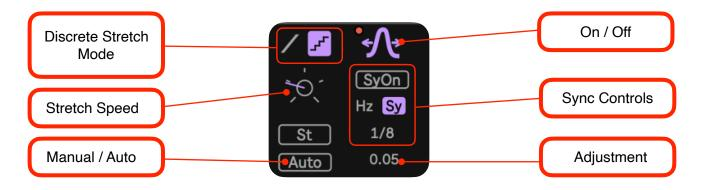
Pigra 2.0's stretch feature allows delay repetitions to slow down or speed up over time.
