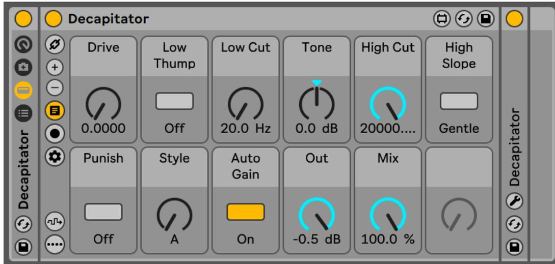
When using the controls in the floating window of the VST plugin, the device controls move at the same time. When using the device controls, the VST plugin controls also move at the same time.
